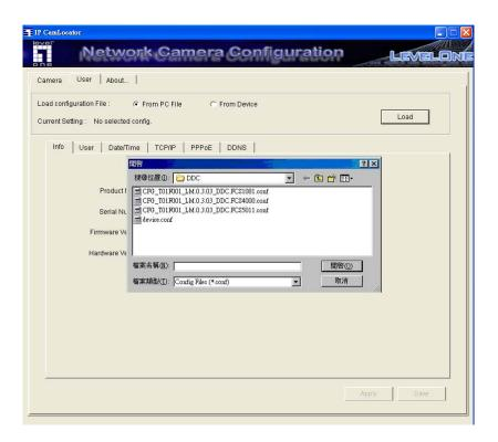
**From Device :** Click it and press **Load** to select the specific device in the network. Type the **Username** and **Password** to load configuration from device.
